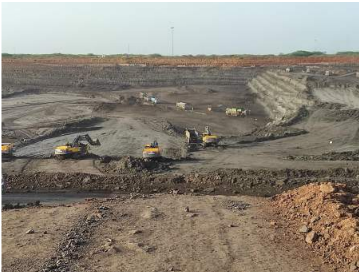
Fig 3.3.1 Mine Pit with Benches
