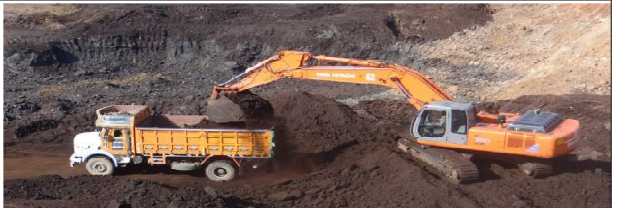
Loading of consumer trucks directly from lignite face
