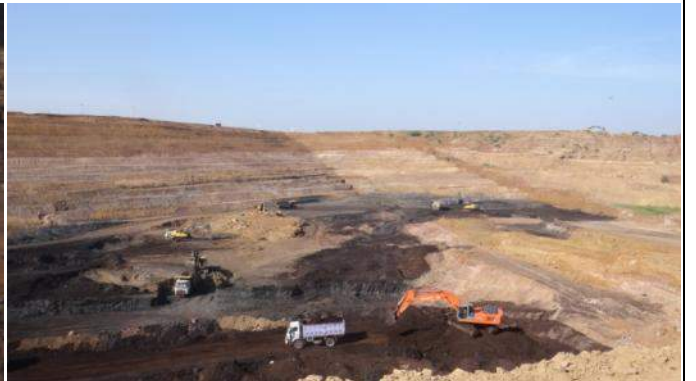
Loading of consumer trucks directly from lignite face
